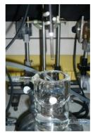
Fig. II.3. Pyrex cylindrical photo-reactor
